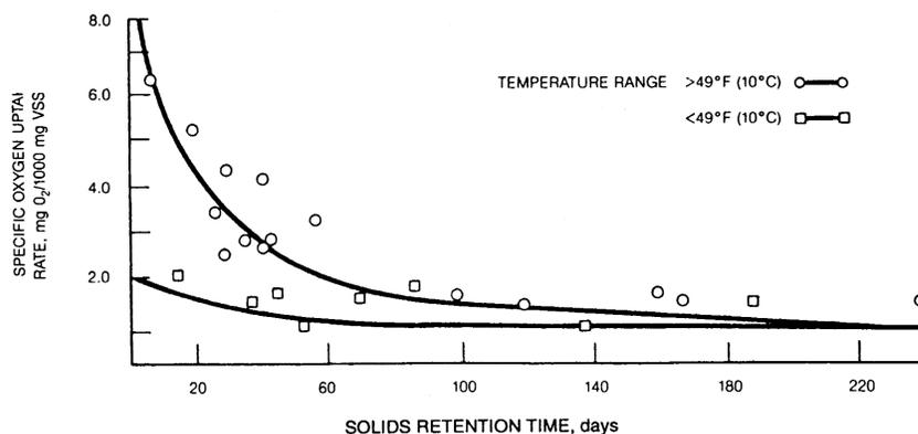
**FIGURE 20.48** Influence of solids retention time and liquid temperatures on the oxygen uptake rates in aerobic digestion.
