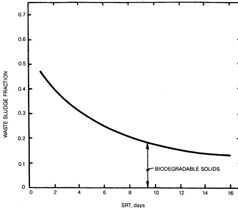
**FIGURE 20.49** Effect of solids retention time on reduction of biodegradable solids by aerobic digestion.
