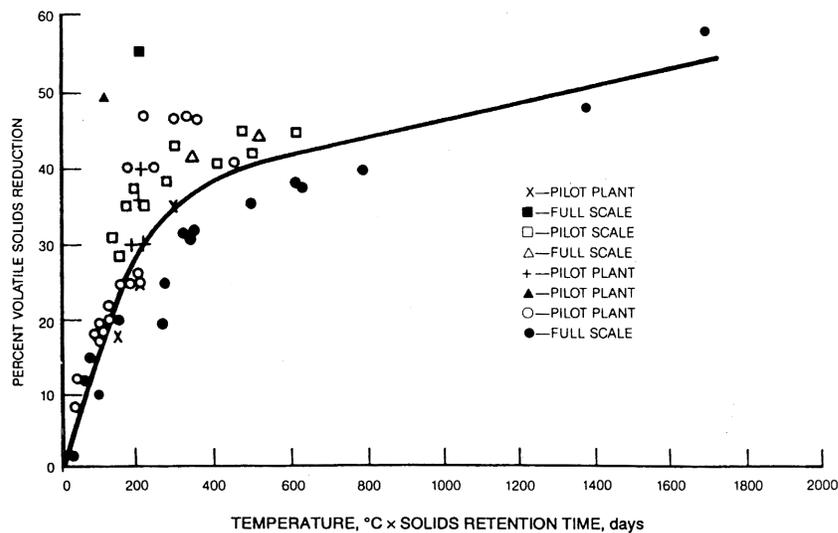
**FIGURE 20.51** Volatile solids reduction as a function of digester liquid temperature and digester solids retention time.
