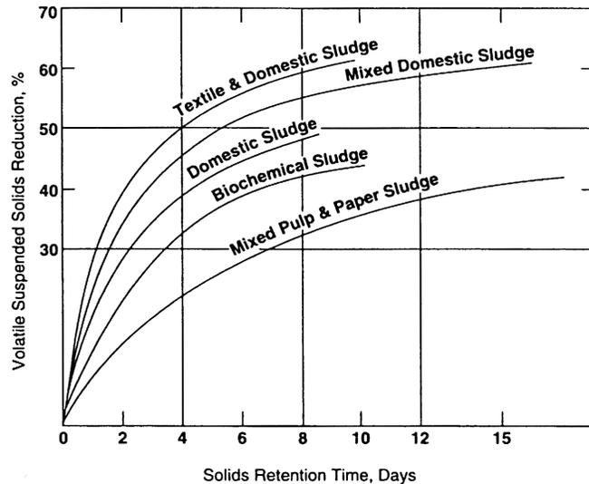
FIGURE 20.50 Relative solids destruction of several sludges by aerobic digestion.
